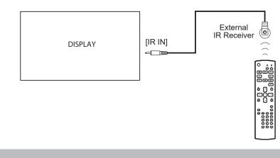
Connect the IR sensor cable to the IR IN connector of the LCD display.
